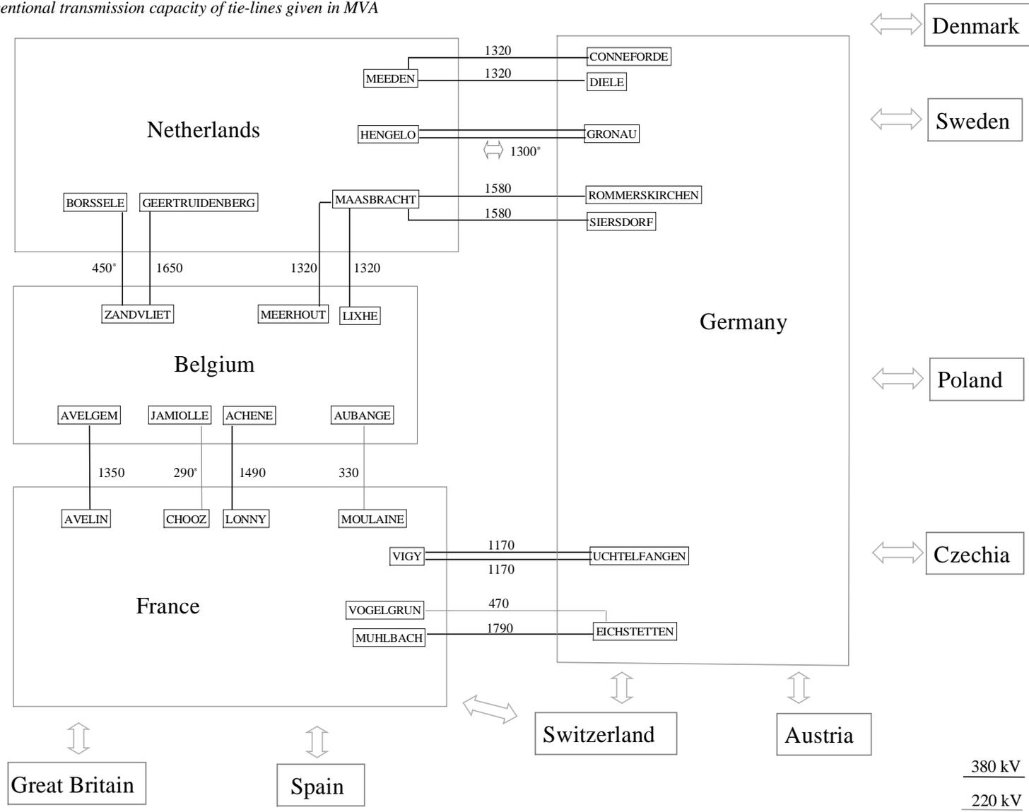
Fig. C.2: Cross-border lines between the Netherlands, Belgium, Germany and France (capacity values in MVA)
