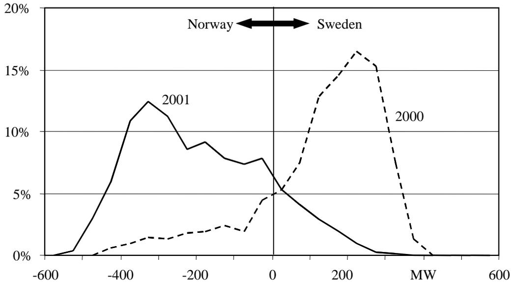
Fig. E.11: Probability density function of power flow on the Nea-Järpströmmen tie line between Sweden and Norway in 2000 and 2001 (source: [www.statnett.no](http://www.statnett.no), data from 4 Apr 2000 until 26 Oct 2001);
