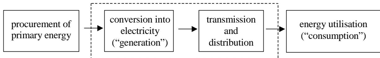
Fig. B.1: Subsystems of electrical power supply
