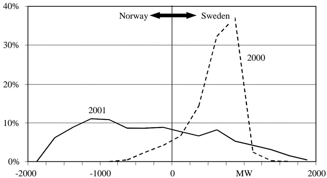
Fig. E.12: Probability density function of power flow on southern border section between Sweden and Norway in 2000 and 2001 (source: [www.statnett.no](http://www.statnett.no), data from 4 Apr 2000 until 26 Oct 2001);
